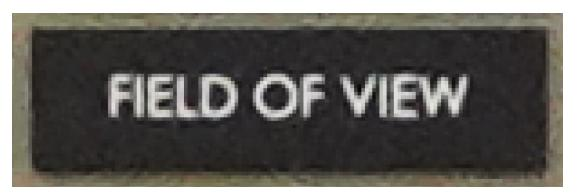
This is in focus, the transition from the light to dark parts of the sign occur within 1-2 pixels
